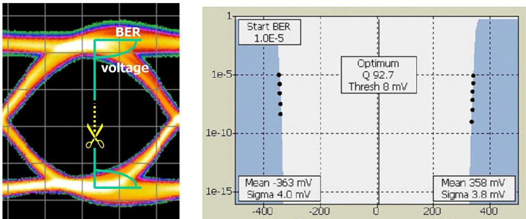
Figure 11 (a), (b). Moving the BERT decision point in voltage to trace out the BER profile of the one and zero levels.
