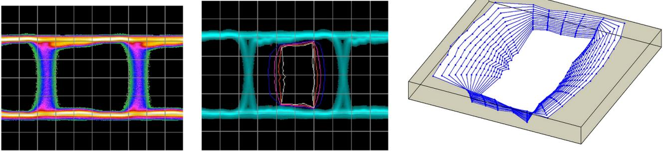
Figure 15 (a), (b), (c). (a) Eye Diagram, (b) BER Contour, (c) Eye Bowl.
