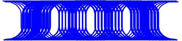
Figure 8. An eye diagram triggered such that the delay between jittered clock and jittered data destructively interferes.
