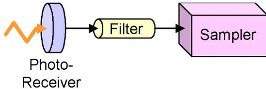
Figure 13. Block diagram of a reference receiver.
